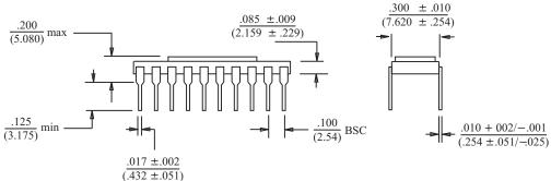
BSC = "Basic Spacing between Centers" is theoretical true position dimension and has no tolerance. (JEDEC Standard 95)
